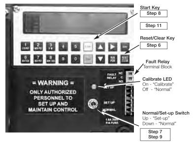
Figure 6. Internal Set Up Switches/Indicators and Keypad/Display Layout
